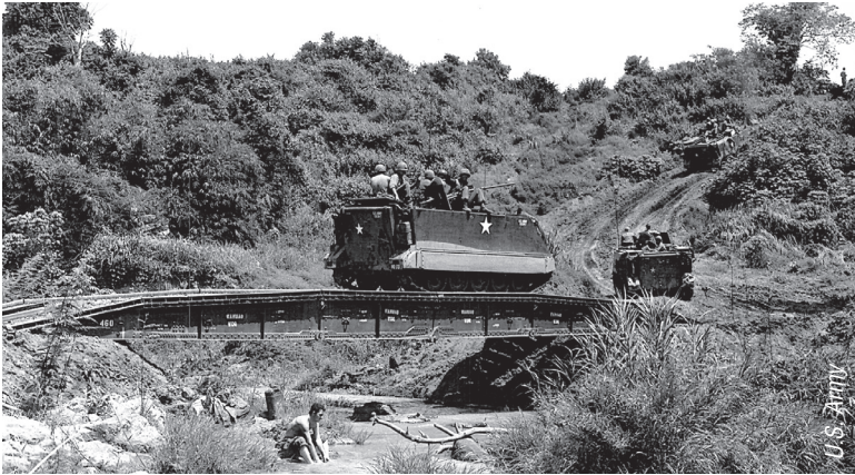
M113 armored personnel carriers assigned to the 1st Brigade, 5th Infantry Division (Mechanized), cross the sixty-foot span of an armored vehicle launched bridge in the Khe Sanh area in June 1969.
