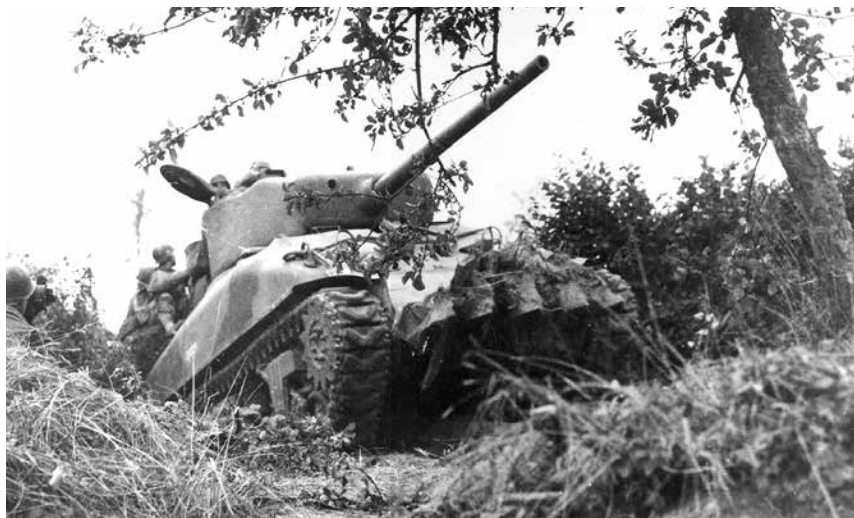
Tank, modified with iron teeth, cuts through the bocage. (National Archives)
