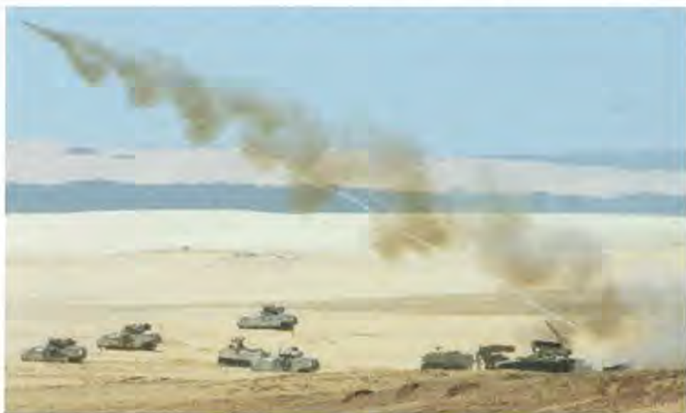
Mine Clearing Line Charge
