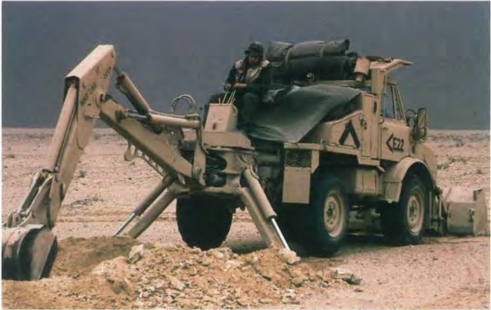
Small Emplacement Excavator; below, Small Emplacement Excavator and Armored Combat Earthmover (Left) Used To Dig Protective Positions for Vehicles and Equipment
