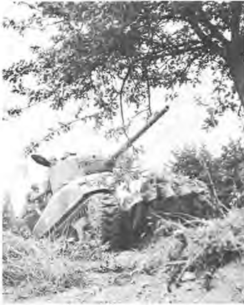
RHINO TANK with hedgerow cutter crashing through a hedgerow.
